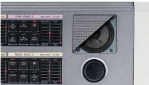
Located to the left and right above the panel. Supplements the stereo effect of the main speakers for the person playing.
