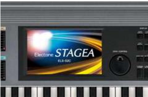
A large, 7-inch LCD touch panel is easily visible from the player's position. Combining it with the data control dial immediately adjacent enables intuitive operation of the controls.
